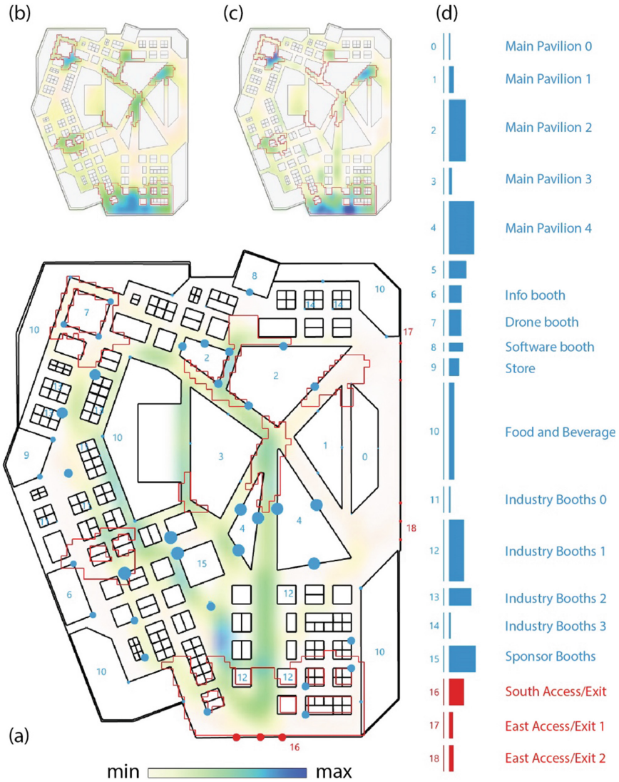
Fig. 7. Productive congestion visualization samples: (a) sample heatmap of productive congestion overlaid on exhibit hall plan layout. Blue and red dots represent respectively sink and source points. Their size reflects assigned weights; (b) heatmap of observed congestion data; (c) Euclidean difference between simulated and observed data; (d) dashboard showing weights grouped by program: of each rectangle, the width reflects assigned weight value, while the height reflects program surface area.
