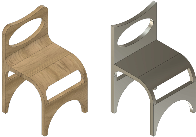
Fig. 3. Modeling operations other than sketch and extrude are suppressed to expand the data quantity. An example design before (left) and after (right) the fillet modeling operation is suppressed.
