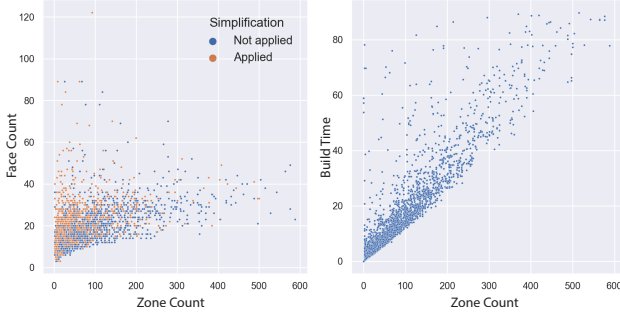
Figure 3: Zone graph construction statistics. (Left) Zone count vs. B-rep face count. (Right) Zone count vs. zone graph construction time (in seconds).
