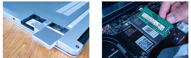
Fig. 5. (a) IO system that allows users to customize the ports on the machine; (b) Memory modules slots.
