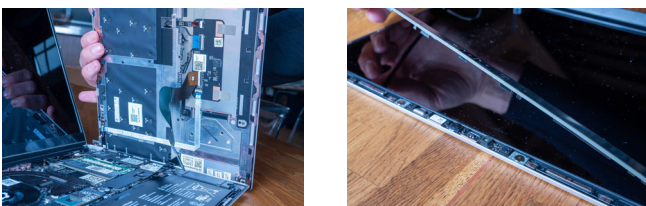
Fig. 4. (a) User-replaceable keyboard; (b) Magnetic removable bezel.
