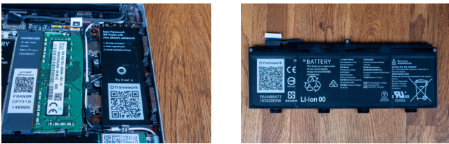
Fig. 3. (a) QR codes for repair guides. (b) Battery repair instructions.
