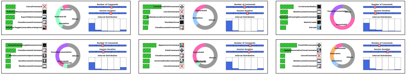
Fig. 2. Examples of Fusion 360 command sequence sessions in the dataset. For each example, the left column shows the top-5 most commonly used commands. The middle column shows the distribution of commands by their category. The right column shows the number of commands and session duration relatively to the overall dataset distribution, as well as the distribution of time interval between adjacent commands where the histogram bin width is 5 seconds.
