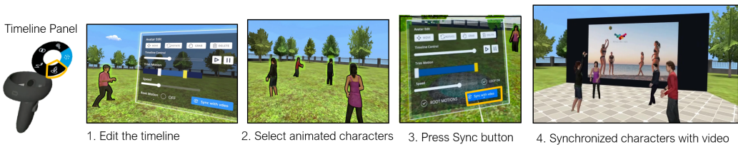
Fig. 6. The timeline panel: users can edit the timeline of an applied motion and synchronize multiple motions with the video timeline.
