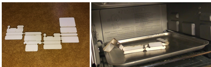
(a) Laser cut layers get assembled into a self-folding laminate. (b) Uniform heating in a toaster oven generates the desired folded geometry.
