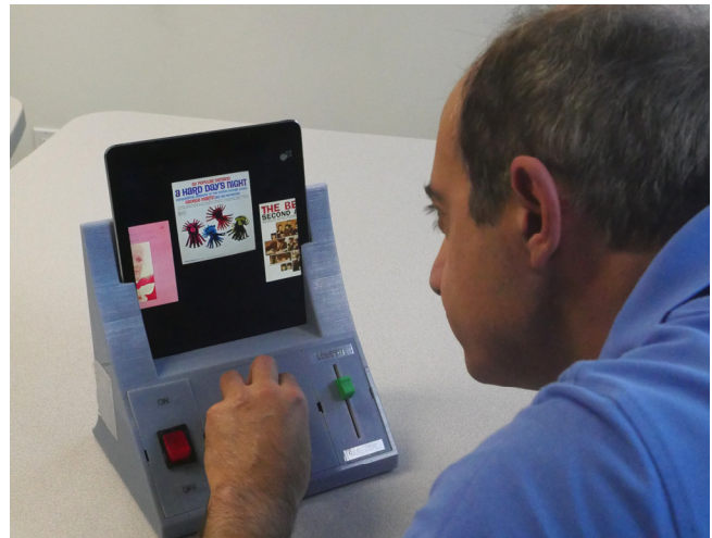
Figure 1: AMI, a reconfigurable tangible music player. By reconfiguring modules in the base, the player can be customized to a user's specific needs.
