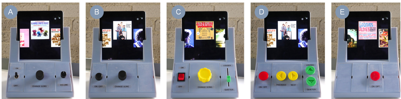
Figure 5: Sample configurations illustrating the adaptability to a variety of needs and use cases of fictitious, simplified personas. These examples serve to highlight how different components may support varied function, and are not meant to be a ‘definitive’ radio for any particular segment of people. The leftmost device may be used by someone without impairments (A), followed by an individual with cognitive impairment (B), visual impairment (C), physical impairment (D), and a combination of multiple impairments (E).
