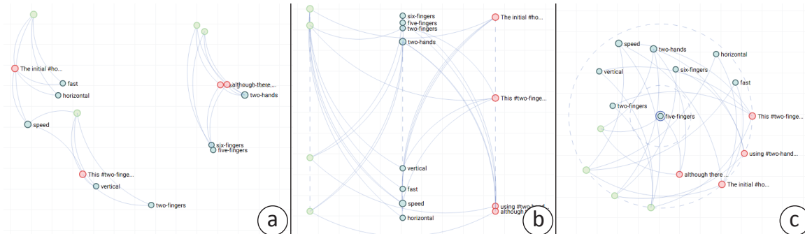
Fig. 1. User-authored annotations are visualized as an annotation graph, including three different layouts a) the projection-plot, b) the slice-plot, and c) the circular-plot, each enabling an analyst to browse the annotation semantics from a different perspective. In the annotation graph, nodes reflect free-form comments (red), short word tags (blue), and their associated data selections (green); links represent relations between annotations. Together, the content and relations of annotations encode annotation semantics.
