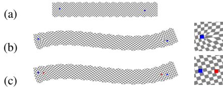
Figure 3: The field (3) moving the vertices in (a) to the locations in (b) creates singularities around the constraints; the Dirichlet solve (4) has a smoother displacement (c), preserving the boundary but relaxing the locations of the constraints to the red points. The solve here uses hard constraints to find \vec{U}^\circ ; soft constraints yield similar singularities.
