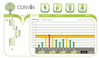
Figure 3. Convia dashboard to monitor energy use throughout a space, zone, floor, or individual workstation in real time.
