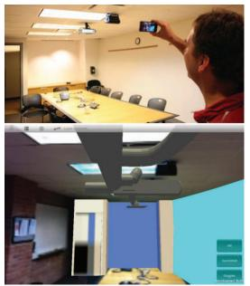
Figure 6. GoBIM app. (top) User holding iPhone to see venting in ceiling. (bottom) Display on iPhone showing what the user sees, including ductwork from the BIM, above the ceiling.
