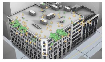
Figure 1. Real-time visualization of an office building with a high density sensor network (sensor icons in green and yellow overlaid on 3D model).
