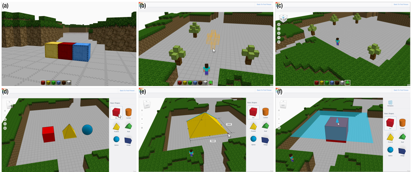
Figure 4. The six stages of functionality in the Blocks-to-CAD system. (a) Minecraft-style block tools; (b) Tree-stamp tool; (c) 3D navigation widgets; (d) Shapes tool; (e) shape-resizing handles; (f) Workplane tool.
