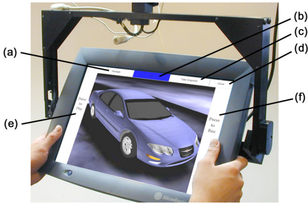
Figure 3. Hand grip and button layout. (a) Flashlight (b) Pen (c) Snapshot (d) Application exit (e) Play (f) Record.
