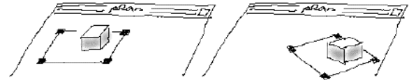
Figure 3. Move and rotate virtual object by manipulating a physical brick, which acts as a handle.
