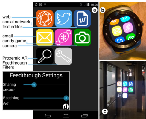
Figure 7. Our homogeneous platform has a similar look and feel on the (a) smartphone, (b) smart watch, and (c) smart glasses. (d) Feedthrough sliders control the extent of information sent and received about device usage.
