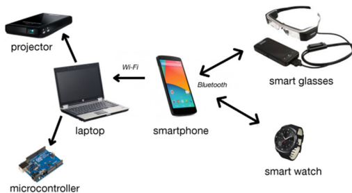
Figure 8. The candid interaction ecosystem links mobile and wearable devices to a laptop, which operates microcontrollers and projectors in our prototypes.
