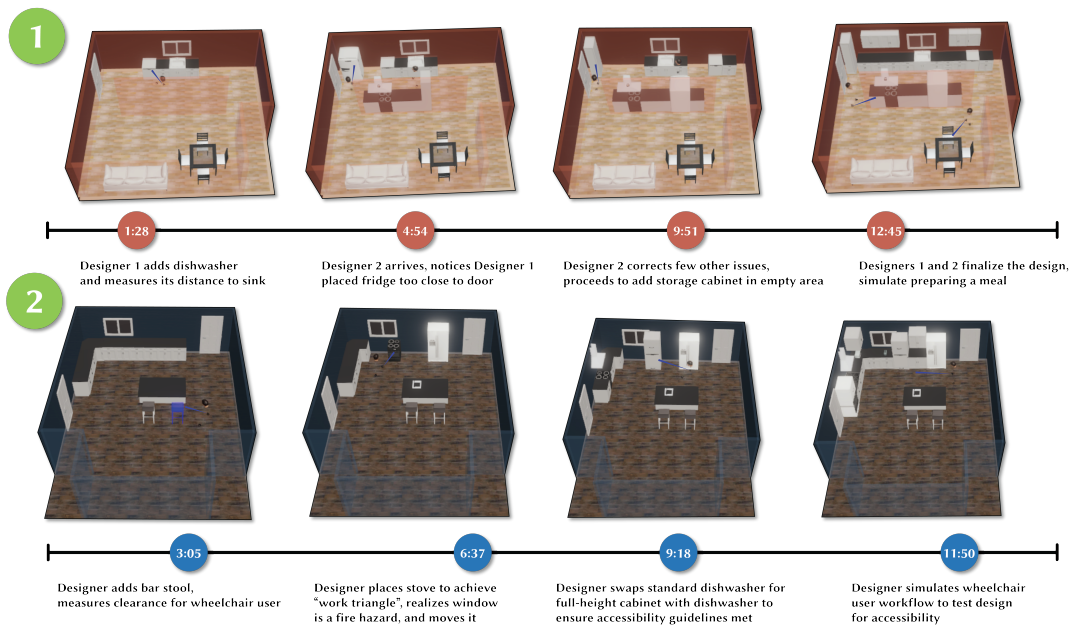
Figure 5: An overview of the spatial design recordings created to help evaluate Tesseract where: (1) is a 14-minutes long recording capturing a designer initially working alone who is later joined by a second senior designer to discuss and review the design; and (2) is a 12-minutes long recording portraying a designer working in a think-aloud fashion to explain their design rationale while designing a kitchen for a client with accessibility requirements.
