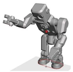
**Figure 3**: Screenshot from a tool implemented in meshmixer to analyze whether an object will be stable under gravity. The center-of-mass (red ball) lies just outside of the convex hull of the ground contact points, so this object will fall over.
