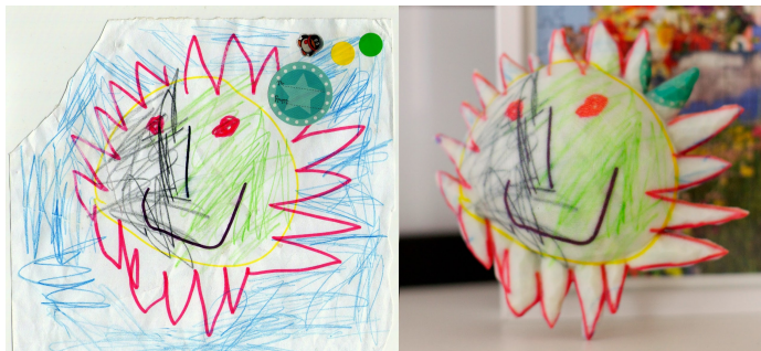
Figure 4: The Crayon Creatures web service allows a user to easily take a child's drawing and inflate it in the third dimension, then create a color 3D print of the result (images copyright © Crayon Creatures, used with permission).
