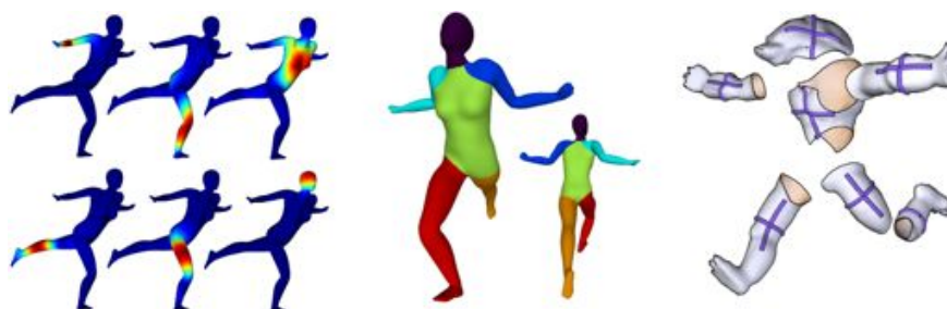
Figure 1: Localized vector fields which are an optimized linear combination of approximate Killing fields (left), a segmentation from these fields (middle), and a decomposition into intrinsic primitives with prominent intrinsic symmetry generators (right).
