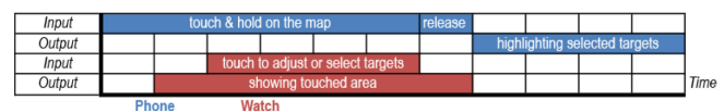
Figure 14. Phrasing between the phone and the watch in a target selection task on a map.
