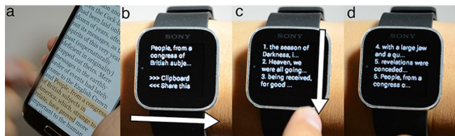
Figure 11. Using the watch as an additional way to copy and paste from a clipboard of text. Selected text (a) is added to the clipboard with a swipe to the right (b), which then displays all the selected text (c). Swiping down goes through the text (c).
