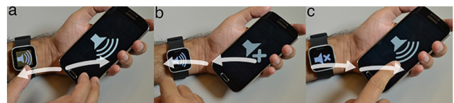
Figure 6. In Email, Multi-device gestures are used to manage new email notifications on both devices.
