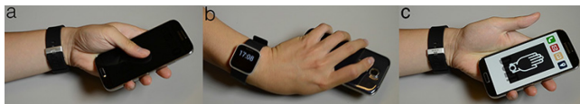
Figure 4. Hold and flip unlocks the phone and registers the devices' spatial configuration (in this case, the watch is worn on the dorsal side of the wrist, also see Figure 2).
