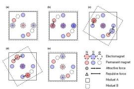
Fig. 5. Sequence of cube-shaped self-reconfigurable robots' spinning. A line square is the electromagnet face of Module A and a dotted-line square is the permanent magnet face of Module B.
