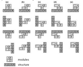
Fig. 11. Basic motion and linear walking using the unconscious traveling algorithm. Modules move clockwise with identical motions.
