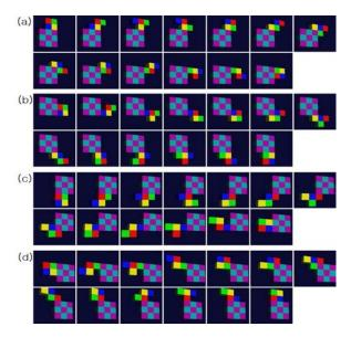
Fig. 14. Snapshots taken from a convex transition using unconscious traveling algorithm simulation. (a) Top-right convex transition.(b) Right-bottom convex transition. (c) Bottom-left convex transition.(d) Left-top convex transition.
