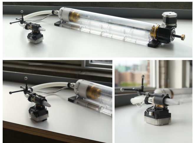
Figure 4. Our custom fabrication machine designed for on-body printing. The machine consists of a motorized clay extruder, a hose, and a hand-held extrusion nozzle.
