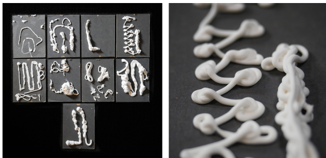
Figure 2. ExoSkin uses a water-based polymer clay as the printing medium.
