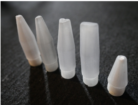
Figure 6. The nozzle tips on the extruder can be exchanged.
