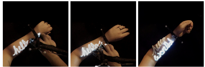
Figure 8. The user holds down the output button and extrudes over the rendered design.
