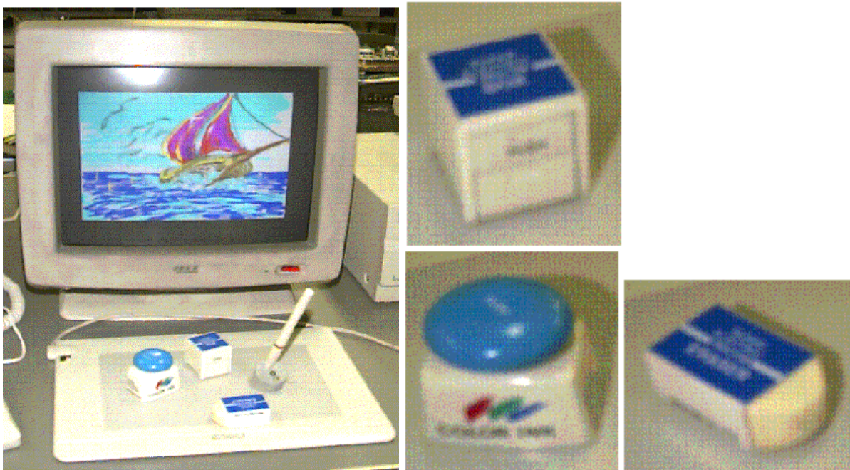
Figure 3.10 A Wacom tablet with prototype "character devices:" a file cabinet, ink pot and eraser.
