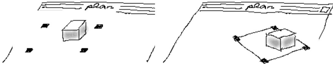
Figure 1.5. Move and rotate virtual object by manipulating physical brick which acts as a handle to virtual objects. Placing a brick on the square selects the object and dragging the brick causes the square to be moved (center of rotation is at the center of the brick).
