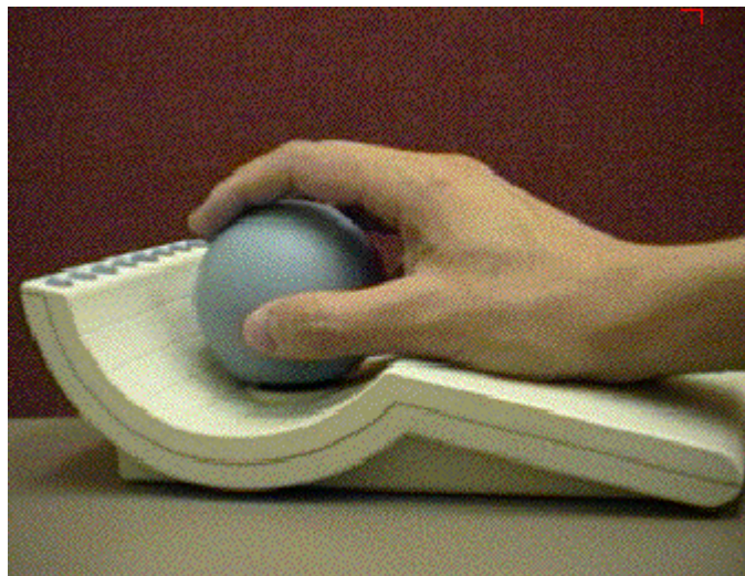
Figure 4.5 The space ball six degrees of freedom input device has a generic physical form well suited for view controls but less so for time controls.
