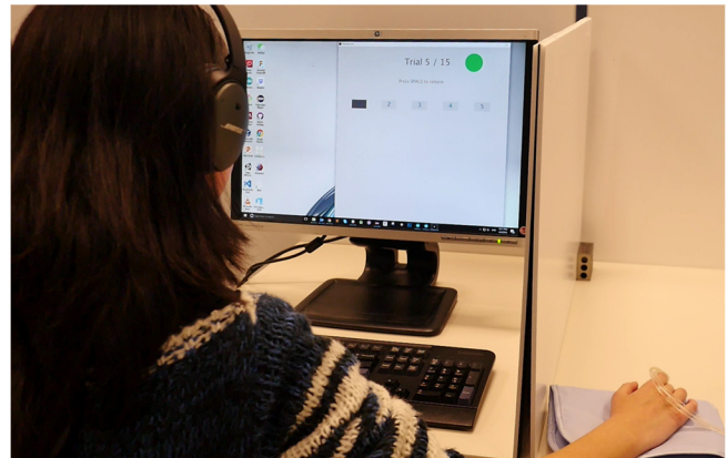
Figure 5: Apparatus for evaluating HydroRing. The user's view of the device is occluded, and they wear headphones to mask the noise of the pumps and valves.
