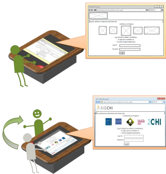
Figure 6: By default, a low-fidelity rendering of each UI component is generated (Top). Once a user walks to an adjacent side of the table, a high fidelity rendering of each component becomes visible (Bottom).
