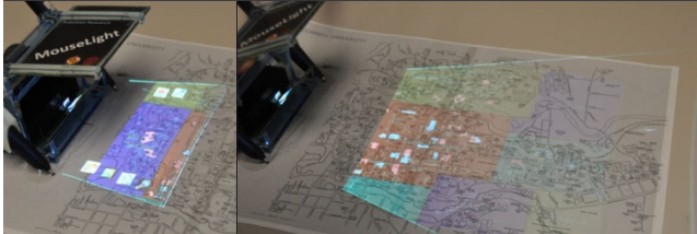
Figure 8 Layer Navigation using Focus/Context button: Users can change the field of view of the projector.
