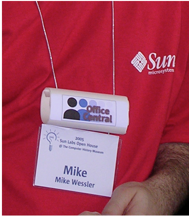
Figure 8. The labels that the RFID tags were affixed to were rolled to keep the tags away from people's bodies. The tags are located directly under the Office Central logo.
