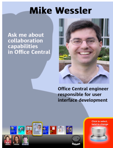
Figure 12. Person ad. One press on the PowerMate initiates an audio connection with the person advertising.
