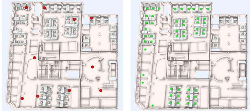
Figure 1 (Left) Position of thermostats shown as red dots. (Right) Sensor-enabled cubicles shown as green dots.
