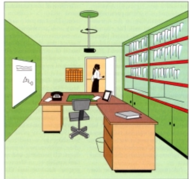
Figure 8. A proposed office environment with a camera mounted on the ceiling for periodically capturing the contents of the office to be stored in the palmtop. The office contains touch sensitive LCD strips (appearing in green) for accessing electronic annotations.
