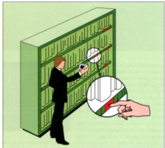
Figure 7. Computer-augmented library. The electronic database of information is situated around the bookshelves; the shelves and books emit navigational and semantic information. Touch sensitive LCD strips run along the shelves to select books of interest to refine the search.
