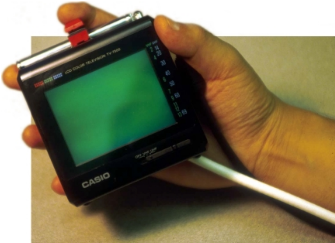
Figure 3. Palmtop unit consisting of a video display, a response button at the top of the unit and a 6D input sensor for providing x, y, and z positional information and organization (pitch, yaw and roll).
