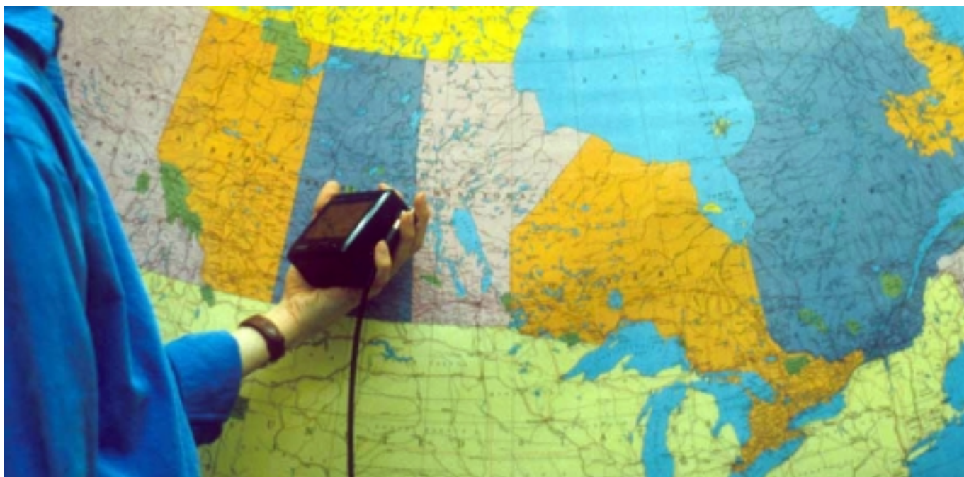
Figure 6. An active map which emits various layers of information is quickly accessed by the palmtop unit. A map of Canada is shown and the user is requesting detailed weather information for a region on the map by moving over the region of interest.
