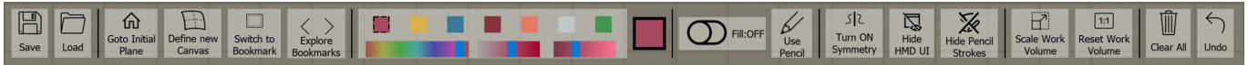
Figure 8. 2D UI toolbar. (left to right) save/load, initial canvas , create canvas , explore and select bookmarks, color tools (palette, HSV sliders, indicator), fill, pencil/ink toggle, symmetry plane, UI and pencil toggles, workspace scaling and reset, clear all and undo stroke. Buttons are shown only if currently useful. For example, selecting the pencil hides color tools. Icons © icons8.com. Used under CC BY-ND 3.0.
