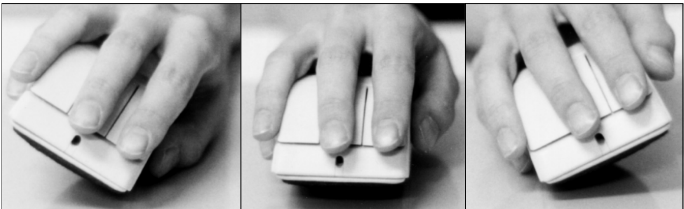
Figure 2. Tilting action of the Rockin’Mouse
