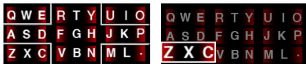
Figure 9. Visual lines help distinguish the characters which require a swipe in one of the side zones. Level 2 shows the selected region in-place, so the entire keyboard is still visible.
