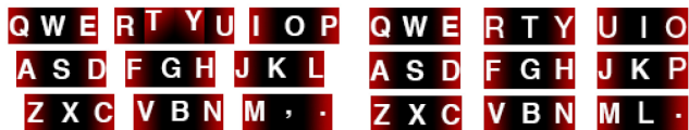
Figure 7. Swipeboard's layout is consistent with QWERTY but has a 4-character group. Our modified layout shifts the locations of 'P' and 'L' so each group has three characters.
