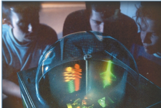
Figure 1. Felix: a dome-shaped swept-volume display. When the volumetric display sweeps a periodically time-varying 2D image through a 3D spatial volume at a higher frequency than the human eye can resolve, it generates an image that the viewer perceives as a 3D volumetric image.
