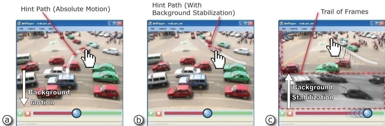
Figure 4: Background stabilization on a scene where the camera pans upwards. (a) The actual motion of a car is hard to perceive by users. (b) Background stabilization presents users with a motion path close to the car's perceived motion. (c) When the car is dragged, background stabilization shifts the video frames and leaves a trail of previously displayed frames.
