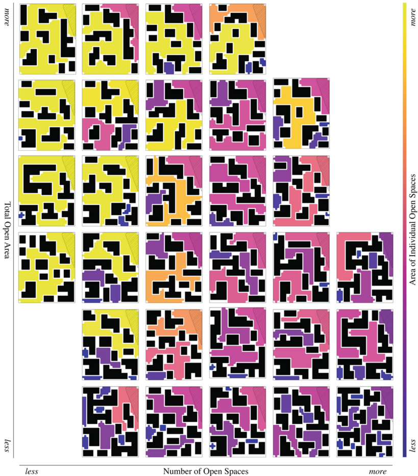
Fig. 9. An example of 3D feature mapping for intuitive navigation of design spaces. Here we show how additional attributes can be extracted (such as number of open spaces and area of individual open spaces) to further aid the design space navigation.
