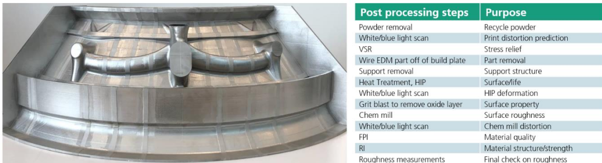
Fig. 5 90° section used for post-processing evaluation (left) and list of post-processing steps (right).
